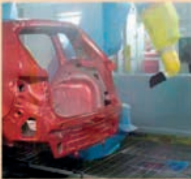
Paint robots at this Volkswagen factory help reduce employee costs, and can be programed to use the minimum amount of paint required.
